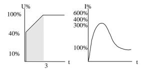
Upon start, the voltage quickly increases to the Initial Voltage value (40% Un) and then gradually ramps-up to nominal.
